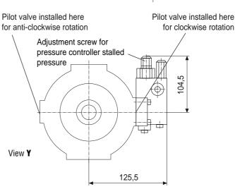
DFR valve, flow controller blocked and not tested
