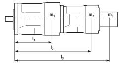
$m_1, m_2 [kg]$ Weight of pump  $l_1$ ,  $l_2$  [mm] Centre to centre spacing
