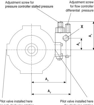
Pilot valve installed here for anti-clockwise rotation
